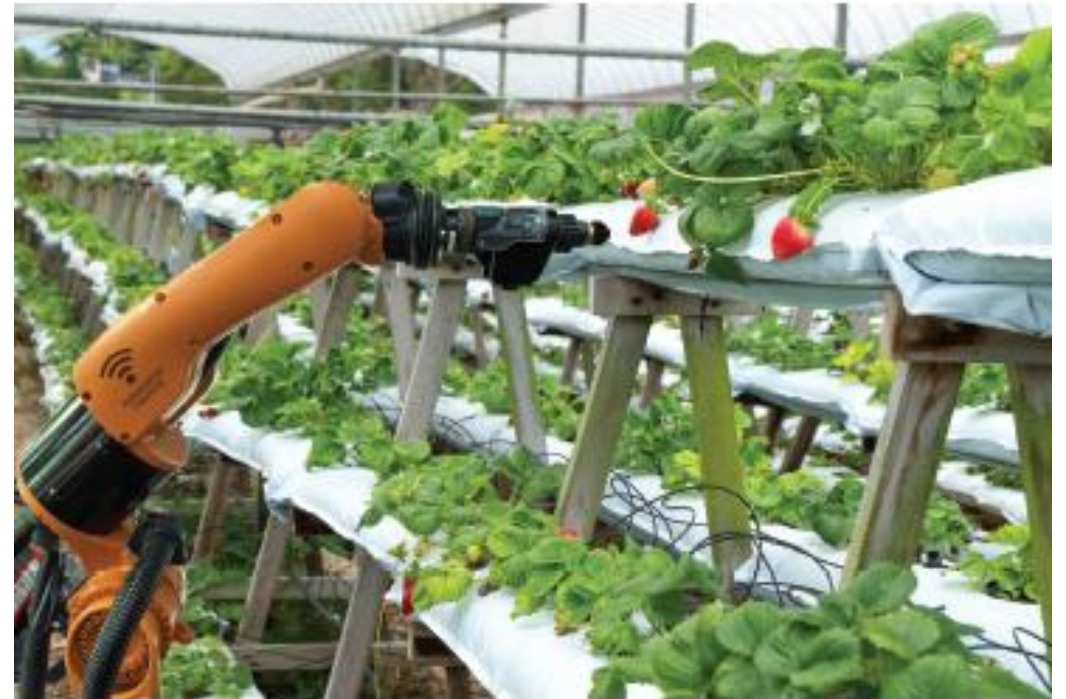
Figure 4-39 Robot used to detect weeds and spray chemicals.
