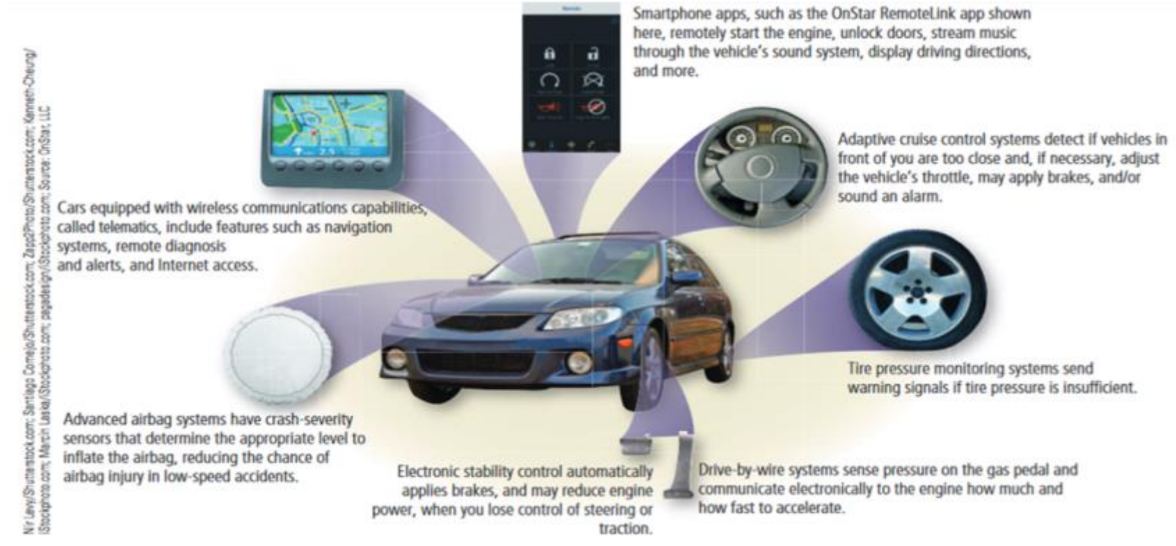
Figure 1-6 Some of the embedded computers designed to improve safety, security, and performance in today's vehicles.
